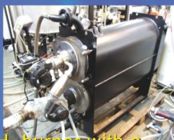
Prototype H 2 burner with a condensing boiler (60 kWth)
